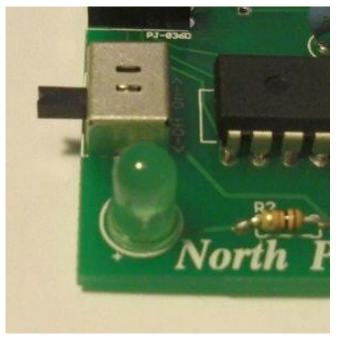
The final step is the LED. If you check carefully, you'll fine that the package has a flat side. The silkscreen on the PCB shows a flat side, simply align the two. Alternately, the silk screen also shows a small "+" on the bottom side of the LED footprint. The longer leg of the LED is positive side and should go through the bottom hole.
