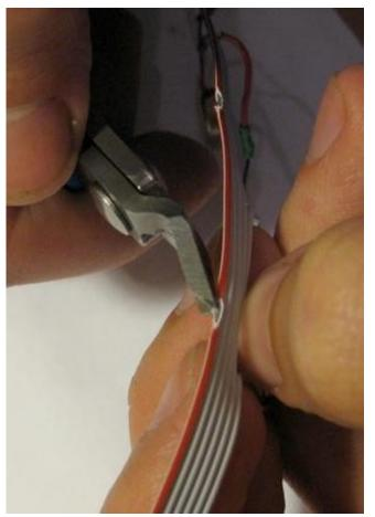
The best way to do this is to take a number of **small**, **gentle cuts** at the insulation with your wire cutters. Once a tiny bit of the metal wire is exposed, stop cutting away and instead use the sharp edge of the cutters to **scrape a bit more insulation away**. After that it can also be helpful to pull at the side of the opening to widen it slightly. If you do accidentally cut the whole wire, don't worry! Just solder it back together.
