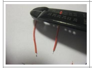
These extension wires should be just **about one inch long**. While you're at it, go ahead and **strip the ends** of these wires. You should have a bit of extra wire in case you mess up, but not too much so be careful!
