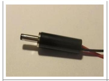
Once both leads are soldered, use pliers to close the strain relief crimp at the end of the outside contact. Then you should be able to slide the cover over the contacts and screw it shut.
