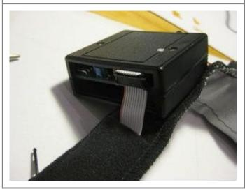
If you have much ribbon cable left over, trim it with some scissors then go ahead and **plug the display into the controller**. Congrats, you should be done building! Slowly turn the North Paw in a circle, and make sure that all eight motors are connected. Put it on and see how it feels!
