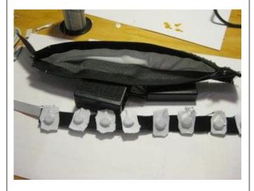
In this, the final step, you'll **stuff the motor array into the armature**, position the controller and battery onto the exterior of the armature, **and hook them all on up together**.
