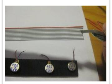
Now you need to start separating **the different strands of the ribbon cable**. The easiest way to do this is to get your wire cutters in between two strands and gently snip the insulation. You only need to snip a millimeter or two, after that you can peel the strands apart by hand.
