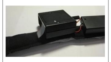
Once the motor array is snug, fold over the left-over length of ribbon cable and pull it through the slit. Now affix the controller to the anklet such that the edge is 0.5 inches from the slit.
