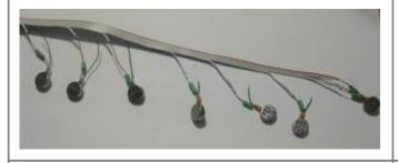
On the very last motor, go ahead and **solder the second lead** to the red (power) line.
