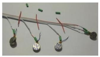
On any short wire motors, **solder on the extension** wires now. You don't need to put the shrink tubing on before soldering this time of course, but it's probably a good habit to do so anyway.
