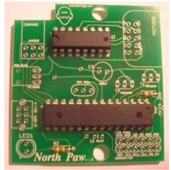
Next do the two ICs. Be careful to get the orientation of the ICs correct – the ATMEGA pin one is to the right, whereas the TPIC pin one is to the left.
