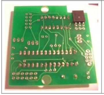
Next mount the  $1\times3$  female header on the \*back\* of the board. The HM55B compass will slot into this later. Solder it tightly in place
