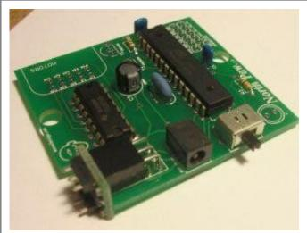
The large electrolytic capacitor is polarized. The stripe down one side is the negative terminal. On the board, the negative hole is marked. The negative side is towards the barrel jack. If you're not sure, compare to the photo.
