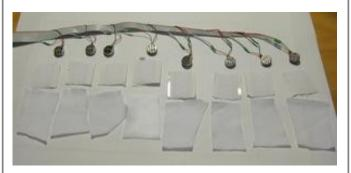
The motors now need Velcro backing so they can be adjustably affixed to the Veltex strip. So, the next step is to cut the long thin strip of sticky-back Velcro into 8 equal pieces. The motors will be sandwiched between these Velcro squares and some thin, stretchy fabric, so take the bit of fabric included in the kit and cut that into 8 equal squares as well.
