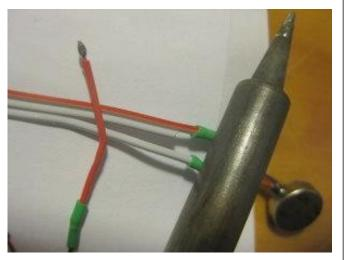
If you don't have a heat gun, you can shrink the tubing with the soldering iron. But, don't go crazy! Gently slide *the barrel* of the iron across the shrink tubing. DO NOT use the tip of the iron, as this can have the unfortunate side-effect of melting the solder under the shrink tubing, ruining a solder joint which you now can't see because it's under the shrink tubing. Fixing that is always a pain.
