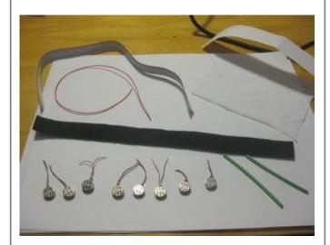
During this step we're building the North Paw's haptic "display". This display consists of **eight vibrating pager motors** attached one by one to a length of **ribbon cable** and mounted on a **Veltex foam backing**. You'll need:
