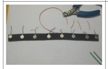
To get things started, place the strip of veltex flat on the table. On top of that, **space the eight motors out evenly**. The motors won't be affixed to the veltex until the end of this process, but having them spaced out on it will be a handy length reference as you cut the ribbon cable.
