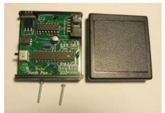
Open up the enclosure bag. You won't need the end panels, but do keep the two screws. Place the PCB into the enclosure (the mounts are not symmetrical, so it only fits properly one way)
