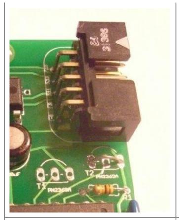
Solder in the motor socket. You'll also need to bypass "T2", which is a switch controlling the actions of motors 1-8. Use one of the leads that you cut off a resistor or cap. Bend it over and solder it between the two outside pins of T2 (see photo).
