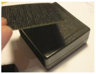
Peel the white backing off the other piece of velcro, and stick it to the non-screw side of the JM22 electronics enclosure. This ensures that if you ever need to open the enclosure up again, you won't have to ruin your velcro. Orient the bare-edged strips of the velcro to run along the closed-face edges of the enclosure.
