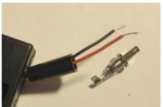
Put the battery wires through the black cover (very important – impossible to do later!). Cut the wires down to  $\sim$ 2 inches in length. Tin the wires with solder.
