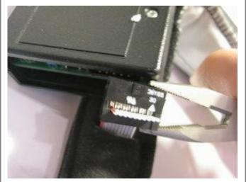
The easiest way to crimp is to hold both sides with pairs of needle nose pliers and squeeze them at the same time. It may take a fair amount of force and the crimp may not snap perfectly; that's ok. If it's holding, it's in well enough and you can squeeze laterally to get the ends to snap. Another way to do this is to set the crimp and cable just right in a vise and turn it shut.
