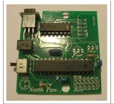
Now solder on the three pin blue resonator (orientation does not matter) and the two 0.1uF caps (orientation does not matter)
