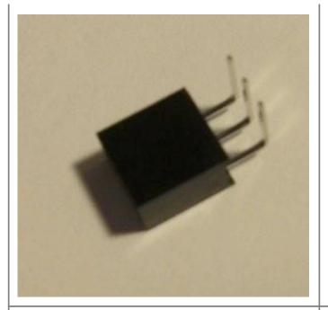
For the other half of the compass socket, you'll need to chop the shorter pins on the  $2\times3$  female header socket. This should leave 3 longer legs. Chop the short ones all the way back – otherwise the little leftover leads could contact the pins from the  $1\times3$  from the other side
