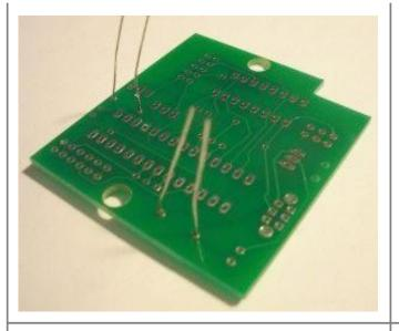
Start soldering with the shortest components first... this makes it easy to turn the board over and solder on the bottom, where nothing is in your way. So we start with the resistors, they are both the same so bend them up and put the through the holes marked R1 and R2 (both are near the ATMEGA footprint)
