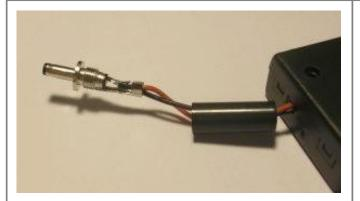
Solder the red wire unto the outside contact, and the black wire unto the inside contact. (yes we know this is backwards, our bad). Make sure not to put any solder/bumps/wires/etc on the outside of the outside contact, as this makes it difficult to get the cover over later.
