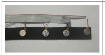
Next **peel back** the lower seven strands until **just to the right** (2-3mm – it doesn't need to be super exact) **of the next motor.**
