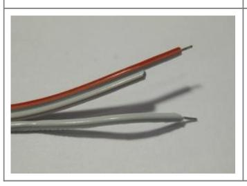
**Strip the insulation off** of all of these wires. For the end two, it might be helpful to cut the second (no connection) strand to keep it out of the way.
