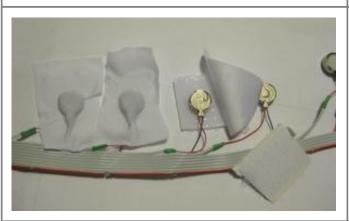
Take the little bits of paper off of the motors to reveal their own adhesive side. Keep that side *up*. Take the paper off of one of the Velcro squares, lift up one motor, and then **push the motor down into the middle of the sticky side of the Velcro square**. Finally, grab **one of the fabric squares, and place that on top**. Push down hard all around the motor so the fabric adheres really securely.
