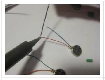
Tin everything in sight. To tin, all you need to do is heat up the exposed bit of metal wire and melt a little solder over it. Don't worry if it seems that the pager motors' little tiny wires aren't picking up too much solder. Also, make sure not to forget to tin both ends of any extension wires you cut.
