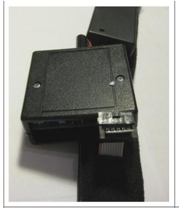
Place the crimp with the notch up and move it to the best position for it plug into the controller. If you look closely you can see the teeth that will be grabbing onto the strands of the ribbon cable and making electrical connections. Make sure these all line up with the strands properly.
