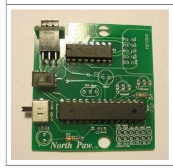
Now do the switch and the barrel connector. For the switch, there are two much larger holes, these will need a lot of extra solder. They provide a firm mechanical hold to the board, so that you can flip the switch without worrying. The barrel connector has two little pegs at the front which should fit into the holes provided.
