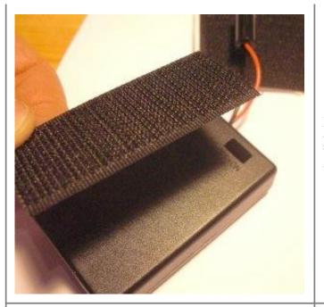
Peel the white backing off the smaller of the velcro pieces, and stick it to the non-opening side of the battery enclosure. This is the side with the (useless) "on/off" labeled hole (as pictured).
